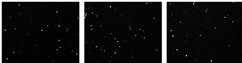
Figure 2. Seal-and-release experiments. An enzyme solution was sealed into the array of femtoliter reaction chambers until a significant amount of fluorescent product accumulated in the reaction chambers. The seal was repeatedly released and sealed, allowing for significant product accumulation after each sealing step.
